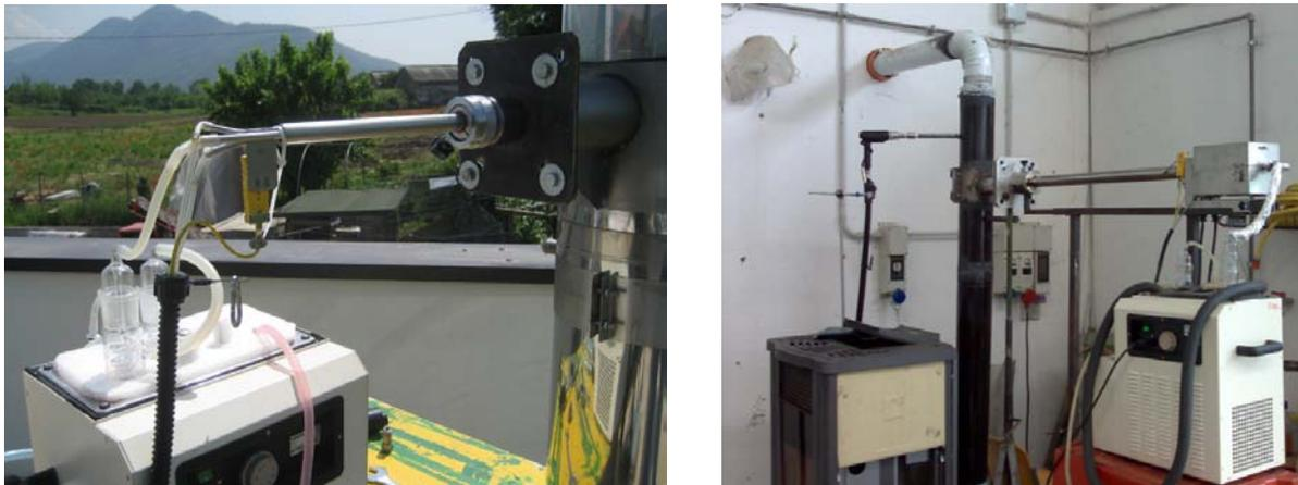
**Figure 2. Ministack probe on boiler chimney (left) and pellet stove (right).**
